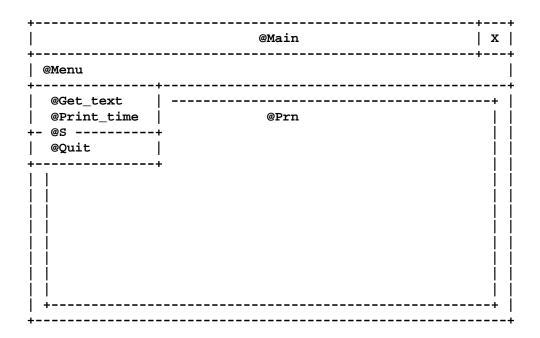
Note that the PRINTER widget, @Prn, actually takes up all the interior area of the @Main PANEL, but it's shown as indented for clarity here.
